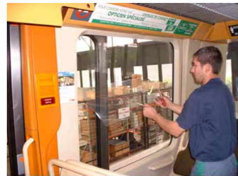
Graffitigard film is easily peeled away when it is vandalised, allowing professional installers to quickly apply a fresh layer.
